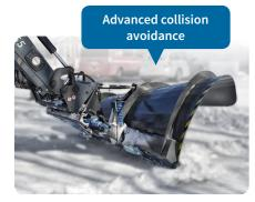
The wing of the Snowek diagonal plows is attached to a spring weighted sledge that moves up and back when hitting an obstacle. This system makes plowing significantly safer.
